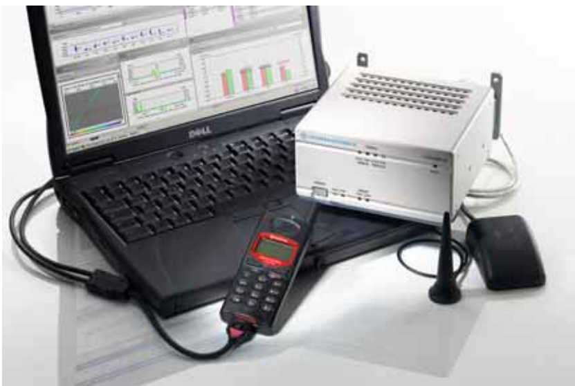
R&S TSMU with a powerful notebook, GPS and UMTS test mobile
